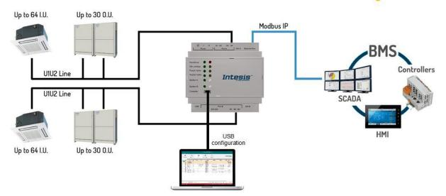
Integration of Panasonic's compatible systems into Modbus TCP systems. 2 Panasonic liness can be connected
