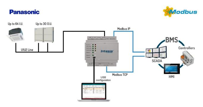
Integration of Panasonic's compatible systems into Modbus RTU and Modbus TCP systems. 1 Panasonic lines can be connected
